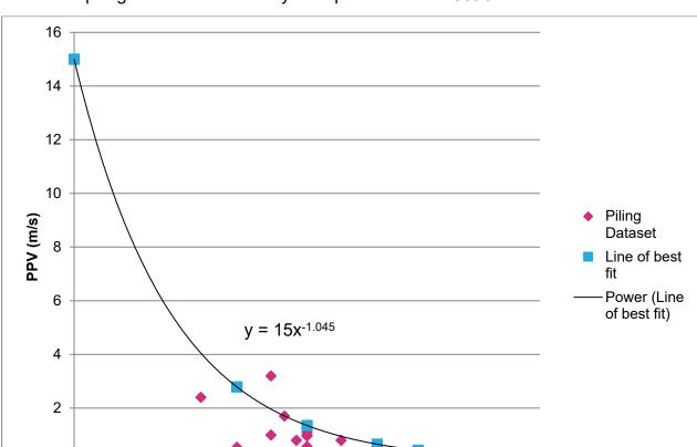
analysis was undertaken to determine a formula for calculating the PPV from piling activities. This analysis is presented in **Inset 5.1**.
